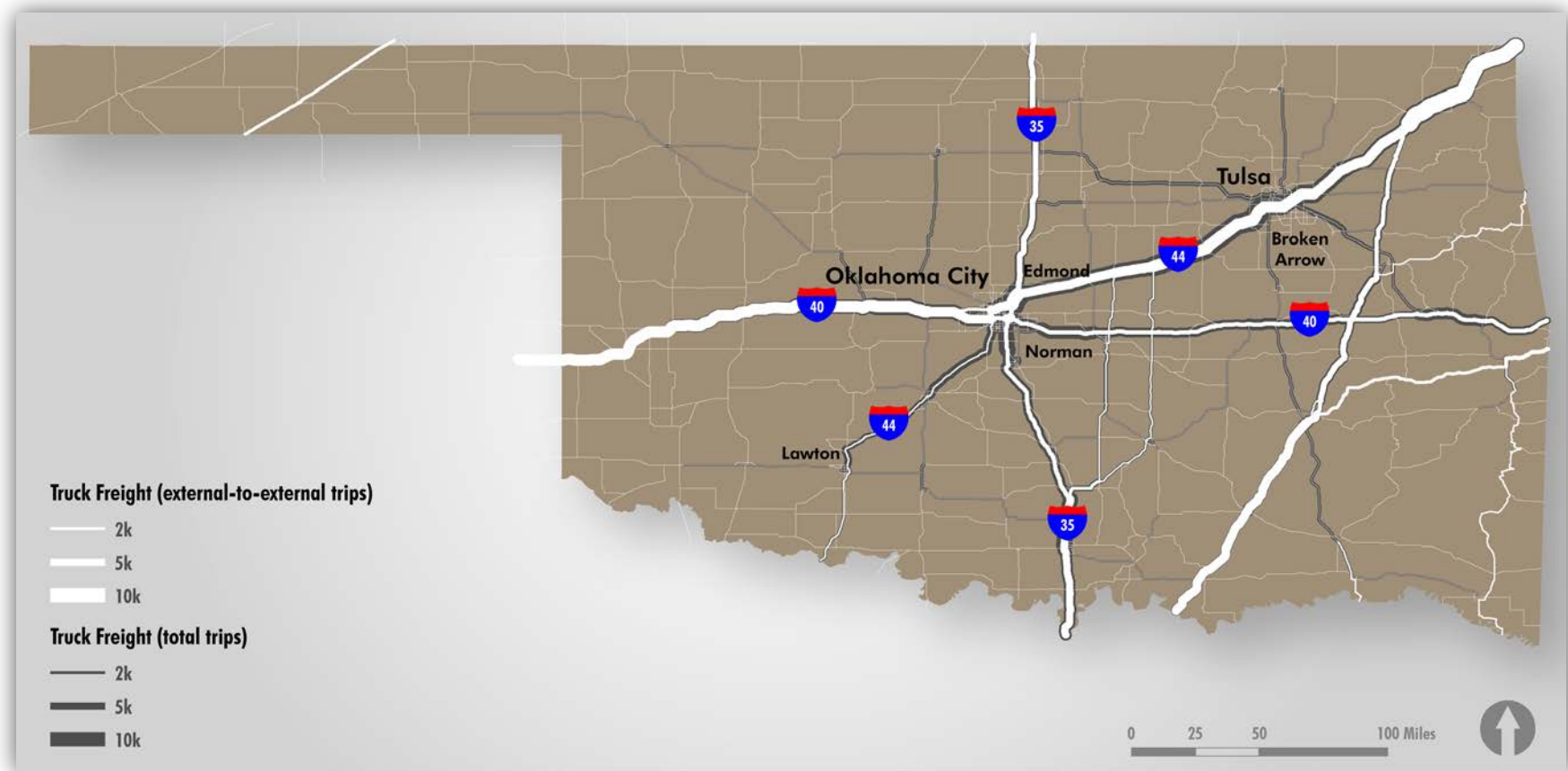
Figure 3. External-to-external (in white) relative to total truck trips in 2009
