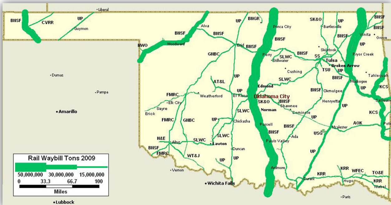
Figure 20. Rail traffic flows on Oklahoma's rail network
